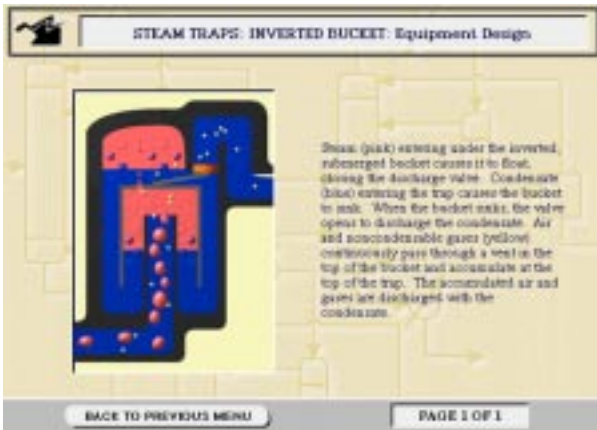
Figure 2. Animation depicting an inverted bucket steam trap in action
