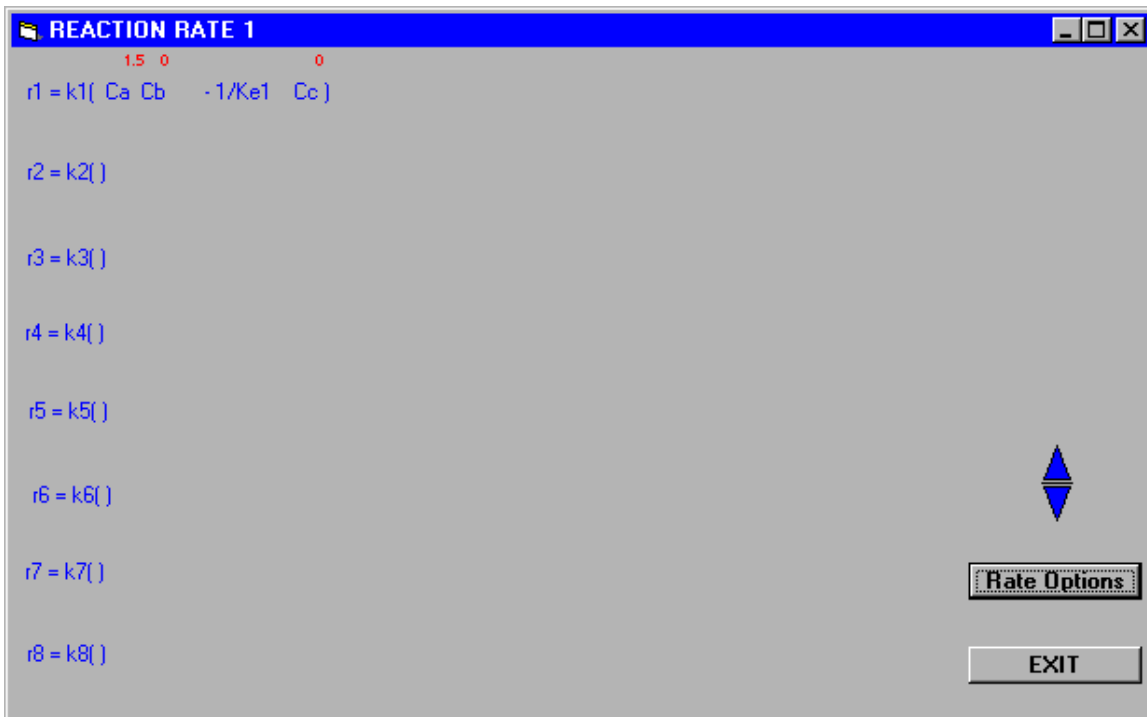
Figure 4. Reaction Rate Input Screen, Example 1, (-r_{1A}) = K_1 C_A^{1.5}
