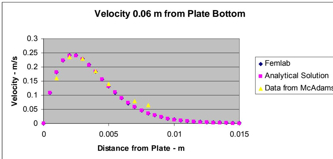
Fig 9. Velocity Profile at 0.06 m
