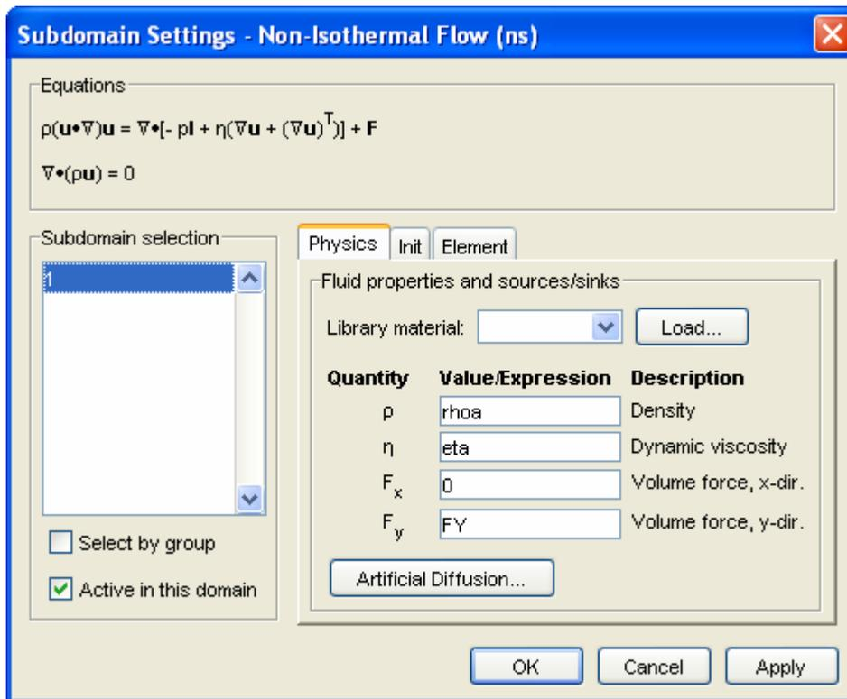
Figure 4 Subdomain Settings – Non-Isothermal Flow (ns)
