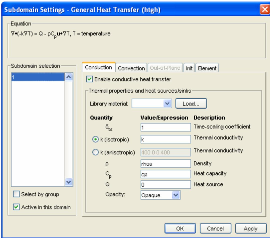
Figure 5. Subdomain Settings – General Heat Transfer (htgh) - Conduction
