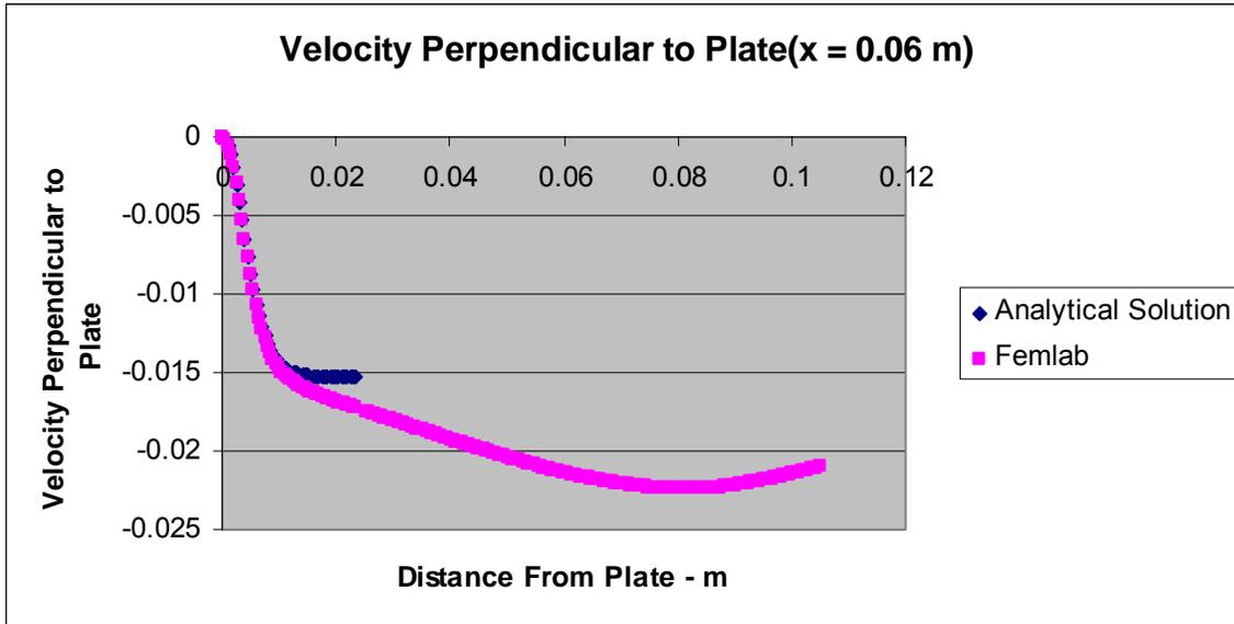
Figure 12. Velocity Perpendicular to Plate
