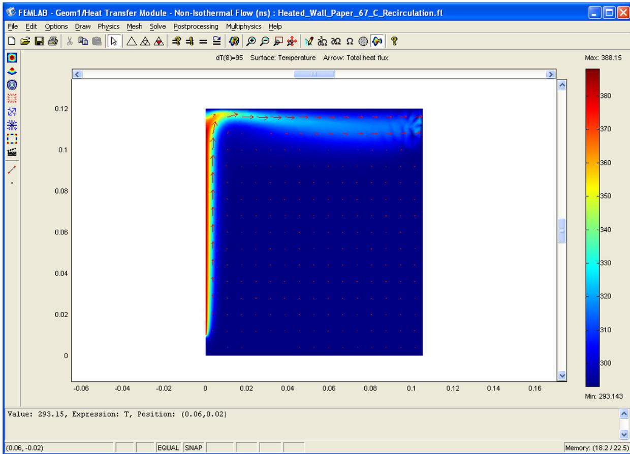
Figure 8. Surface Temperature and Arrows Showing Flows
