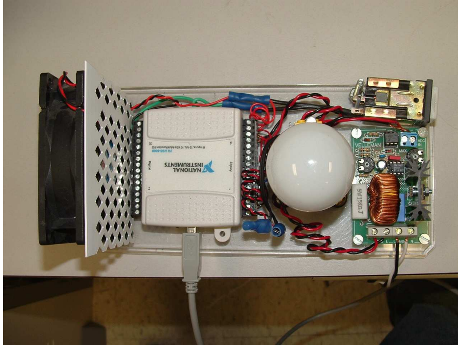
Figure 1: Photograph of the Low-cost Temperature Control Light-bulb Experiment (top view)
