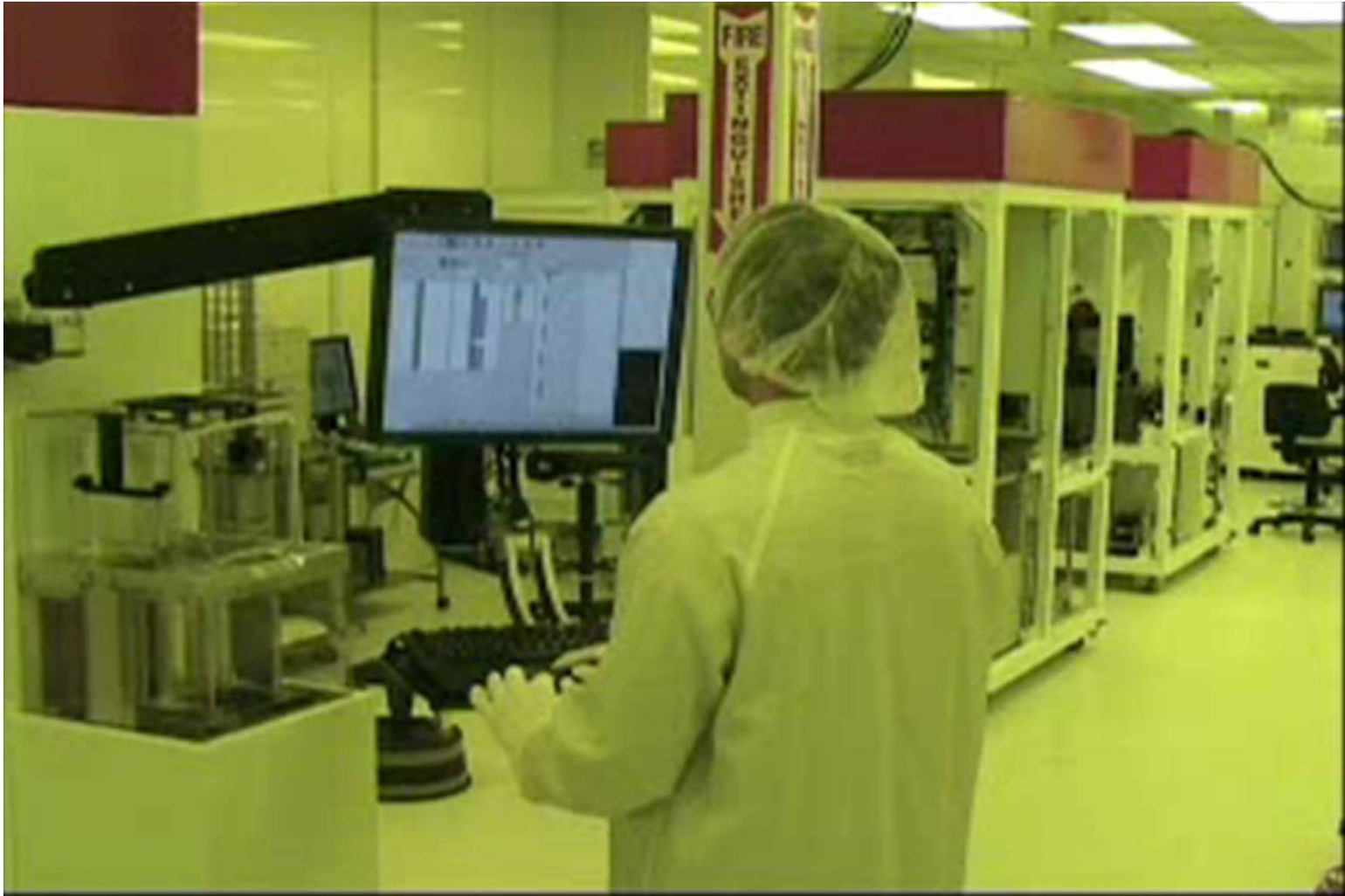
Imprio HD2220 at Molecular Imprints, Austin, TX For High Density Patterned Magnetic Media
